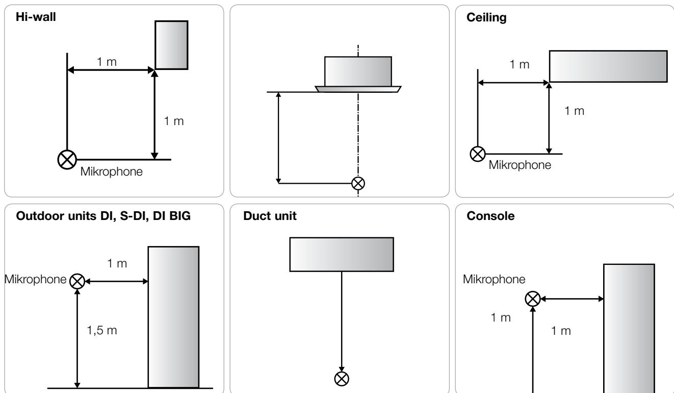
**Sound pressure level:** measured in about 1,5 m distance\* to the indoor unit and 1 m distance to the outdoor unit
