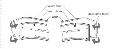
Insert the fabric into the top and bottom side of the air inlet grille.
